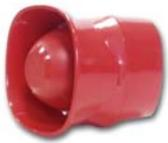
The 24Vdc Symphoni Sounder is a general purpose internal sounder, available either as a very high output sounder for noisy areas, or a high output low current sounder for applications where power is limited. Both versions share the same horn and backbox which has double cable entries for ease of installation.
