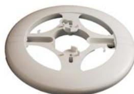
The 4B-6A 4" to 6" Adaptor is designed for use with U.S. style 6" electrical back boxes and provides a flush architectural trim between the electrical box and the 4B-C 4" continuity base. It can also be fixed directly to a ceiling and used to conceal marks left when older, large diameter detectors are replaced with MZX Technology.
