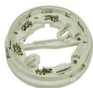
The 4B-D Continuity Base is a standard 4 inch base fitted with a continuity diode, for use with all Series 600 detectors. The base is designed to ensure that conventional systems meet the requirements of BS5839 Pt:1 for callpoints placed after detectors.
