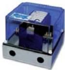
The MT series of enclosures provides a simple, effective means of mounting and protecting MTL700 Series barriers in safe areas or low-risk hazardous areas. Three lightweight polycarbonate enclosures with see through lids accommodate up to 2, 5 and 12 barriers in the safe area. All the enclosures are supplied ready fitted with a nickel plated brass busbar mount, so barriers can be installed and wired up immediately without special tools.
