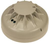
Complimenting the range is the heat sensor which can operate in fixed temperature and rate-of-rise modes with a number of approved sensitivities. It is most often used in areas where high levels of dust are present or where the environment precludes the use of smoke detectors.
