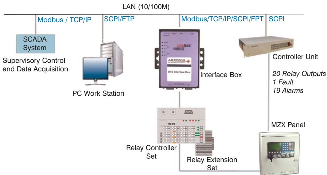
*By means of the Relay Controller Set and the Relay Extension Set an additional 256 relays per sensor cable can be connected.*
