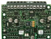
The DDM800 provides the ability to connect and interface 2 zones of conventional 2 wire fire detectors or two 4-20mA sensors to the MX Fire alarm controllers.
