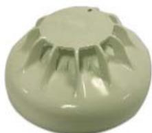
These detectors use two networked thermistors in a bridge configuration to provide a fast response, that depends both on absolute temperature and notes the change of temperature. The rate of rise/fixed temperature heat detectors can be used in areas where smoke sensors are unsuitable due to environmental conditions (smoke, dust etc.). Such areas include kitchens, locker rooms, canteens, garages, loading bays etc.
