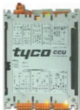
The CCU3/C-MX Bridge enables the direct connection of an MX Technology® fire controller and Minerva® 16E or 80 fire controllers via the H-Bus Communications Driver Module (CDM). No network cards are required in this configuration. The CDM attaches on to the Minerva® H-Bus and provides a serial port for the CCU3/C-MX bridge.
