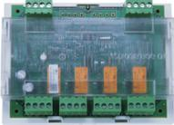
The Quad Monitored Output Module connects directly to the MZX Digital loop and requires a 24Vdc or 48Vdc power supply. It provides four monitored outputs for connection to conventional sounder circuits or auxiliary relays.
