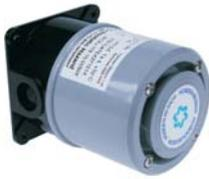
The IS28 Mark 5 Banshee Electronic Sounder is the industry standard intrinsically safe sounder for use in hazardous gas and dust environments. This traditional high profile Banshee Electronic Sounder has 32 tones providing ultimate flexibility and is designed to be connected directly to the 24Vdc sounder circuit of an addressable Fire Alarm Control Panel via an MTL5525 Safety Barrier.
