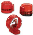
This low power LED beacon is designed to be retrofitted to existing Banshee electronic sounders. Easy and fast installation typically 3 min. Low power 6 mA max at 24 Vdc. High Output LEDs.
