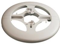
The 4B-6A 4" to 6" Adaptor is designed for use with U.S. style 6" electrical back boxes and provides a flush architectural trim between the electrical box and the 4B-C 4" continuity base. It can also be fixed directly to a ceiling and used to conceal marks left when older, large diameter detectors are replaced with MZX Technology.
