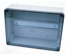
A polystyrene/polycarbonate IP66 rated housing prefitted with a din rail for mounting either 1 x Quad Input/Output Module (QIO850), or 1 x Quad Monitored Output Module (QMO850) or 1 x Quad Relay Output Module (QRM850) complete with a transparent front cover.
