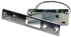
A microswitch lock keep can be used with a deadlock to provide a signal to the panel to ensure that the extinguishing system is only put into Automatic mode when the door is locked shut.
