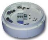
The 600 Series relay base provides dual relay contacts for signalling external devices on conventional detection systems. Very low operating current even when the relay is energised, enable the relay base to be used without additional power. The relay contacts operate when the detector enters the alarm condition.
