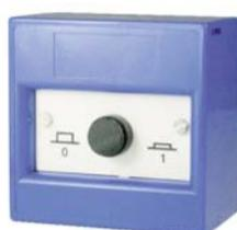
A manual hold call point with activation and end of line resistors making it compatible with the Prescient III Suppression Panel. Operation is via a non-latching push
