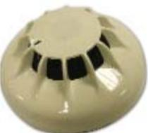
These detectors are capable of detecting the visible smoke produced by materials which smoulder or burn slowly, i.e. soft furnishings, plastic foam etc.; or 'smoke' produced by overheated but unburnt PVC. These detectors are particularly suitable for general applications and areas where cable overheating may occur e.g. electrical services areas. The novel design of the asymmetrical sampling chamber and signal processing techniques stop unwanted alarms caused by very small insects. i.e.
