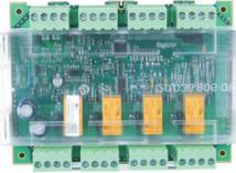
The Quad Input/Output Module connects directly to the MZX Digital loop and provides four change over relay outputs, four High Voltage Relay (HVR) outputs and four monitored inputs. It is loop powered and therefore does not need a power supply, however it can monitor the presence of a local 24Vdc or 48Vdc power supply.
