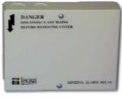
Metal boxed heavy duty alarm relay with 25A mains rated DPCO contacts. Available with either a 240VAC 12mA or 24VDC 50mA rated coil. Suitable for heavy duty switching applications.
