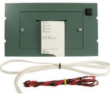
The PRN800 Printer Kit is designed for use with the designer range of MX Controllers (MX4000 and T2000). It is fitted to the front cover of the MX battery housing and is powered from the PSU830 power supply via an FB800 fuseboard in the MX Controller housing.
