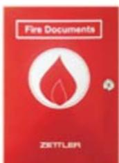
An A4 sized box ideal for the safe keeping of important fire system documents and log books. Formed from red powder coated steel with a cam lock. The box is branded Zettler with a white FIRE logo. 2 Keys are provided and all units are keyed alike. Dimensions 300 x 235 x 50 mm HWD
