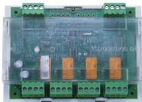
The Quad Relay Output Module connects directly to the MZX Digital loop and provides four change over relay outputs or four High Voltage Relay (HVR) outputs. It is loop powered and therefore does not need a power supply, however it can monitor the presence of a local 24Vdc or 48Vdc power supply.
