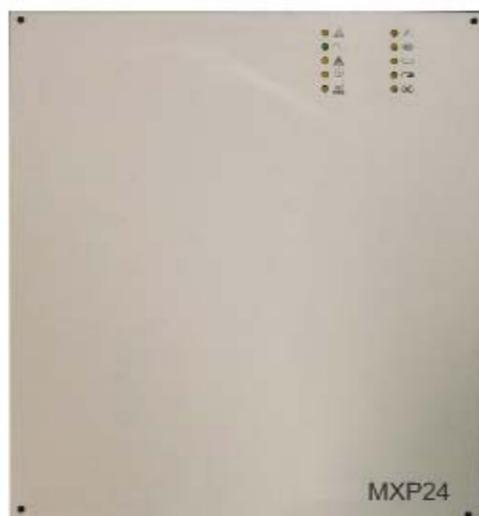
This PSU is approved by IMQ to EN 54-4:1997 + A1:2002 and EN60950-1:2001. The steel housing contains a 5 amp switch mode power supply and monitoring board and has space to accommodate 2 x 12V 17Ah sealed lead acid batteries. The 10 front panel LED's comprehensively indicate the status of the unit.
