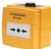
A manual suppression release call point with activation and end of line resistors making it compatible with the Prescient III Suppression Panel. Operation is by break glass.
