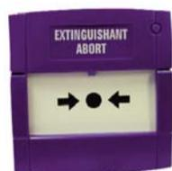
A manual abort call point with activation and end of line resistors making it compatible with the Prescient III Suppression Panel.
